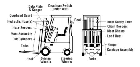
What should an operator inspect during the operational preuse check?
