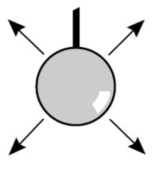
**Indirect light fixtures** distribute 90 to 100 percent of the light upward. The ceiling and upper walls must be clean and highly reflective to allow the light to reach the work area. They provide the most even illumination of all the types of fixtures and the least direct glare. Indirect light fixtures are usually used in offices.
