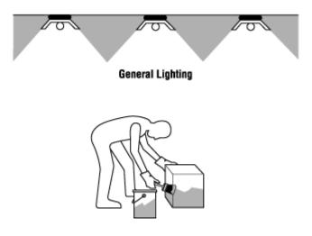
Localized or general lighting uses overhead fixtures in addition to ceiling fixtures to increase lighting levels for particular tasks.
