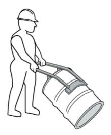
• Use a tilting drum stand to move emptied barrels and drums.
