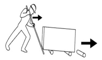
Use rollers positioned at an angle to redirect the load smoothly. This technique reduces the need for manual repositioning.
