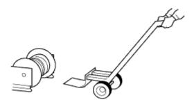
Lever on wheels lifts and moves coils.
