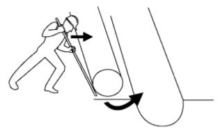
• Use "Come-Alongs" to move a heavy load. Make sure the load is fully on the skid to prevent drag or resistance.
