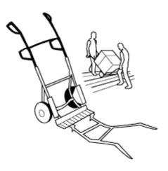
• Use a pump truck to move materials stored on pallets.
