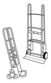
• Choose a sturdy frame hand truck with larger wheels to move materials in rough terrain. An additional set of handles allows for assistance.
