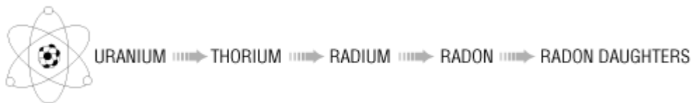
Figure--Production of radon and radon progeny from uranium
