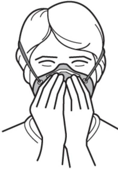
Figure 5: Seal check with a disposable respirator
