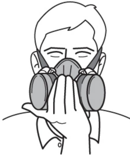
Figure 4: Positive pressure fit check
