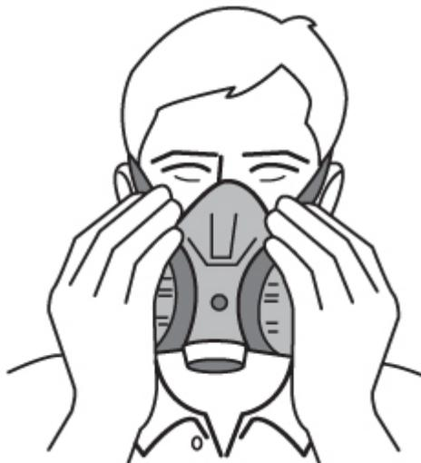
Figure 3: Negative pressure fit check
