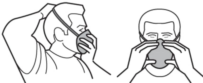
Figure 2: How to put on a disposable respirator
