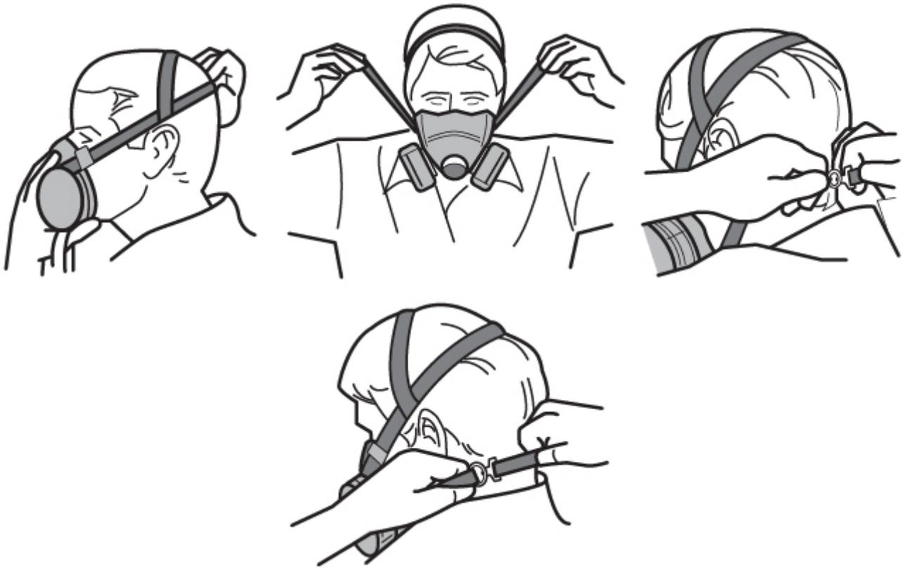
Figure 1: Procedure for putting on a half-facepiece respirator
