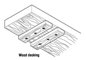
• Only cleat planks at the ends to prevent lengthwise movement. Wiring down planks can also prevent movement, provided the wire does not create a tripping hazard. Where planks overlap, rest the cleated end on the support. Do not use cleats elsewhere on the plank to prevent splitting.
